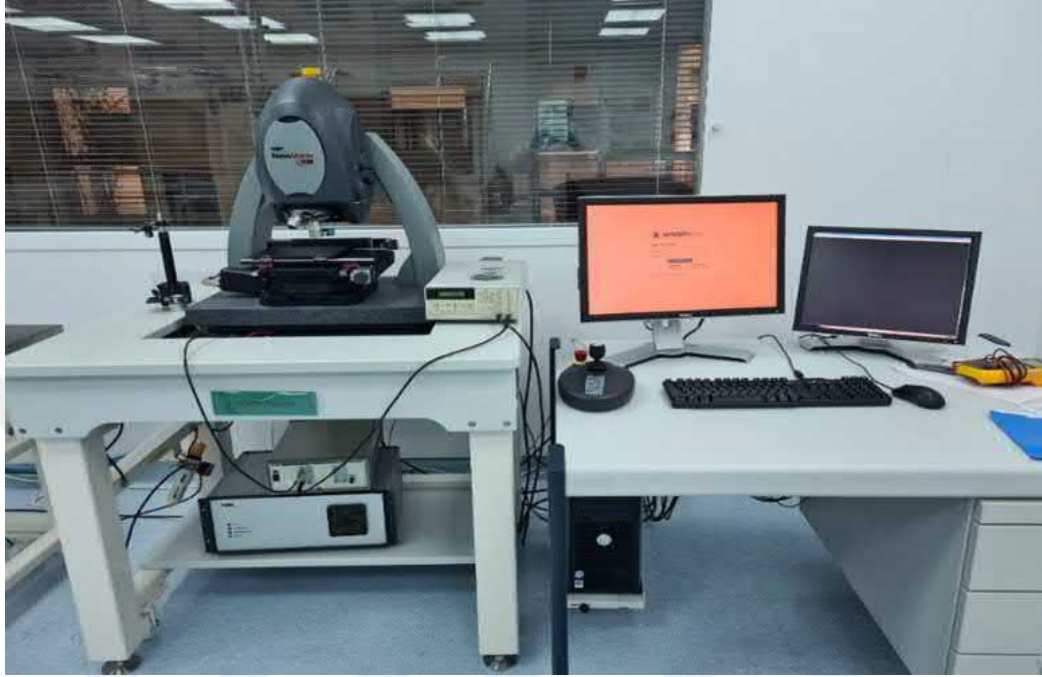
Figure 4.3: Complete setup of the ZYGO Optical Profilometer dynamic measurement
