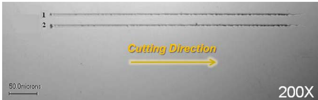
Figure 9.4. Scratches done with (2) and without laser heating (1).
