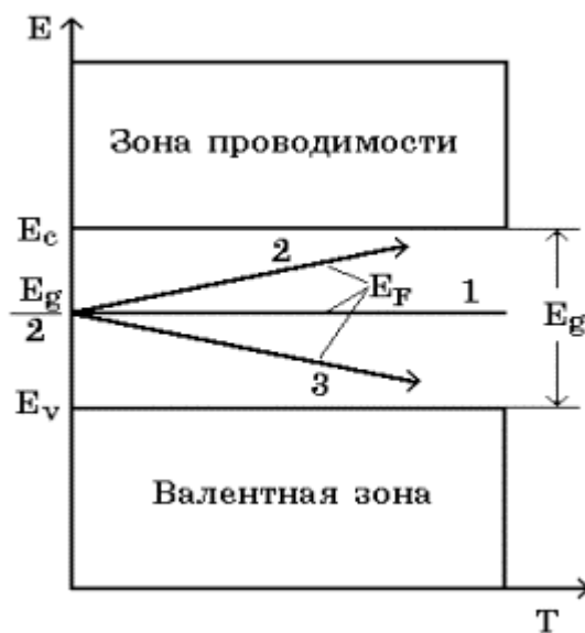
Figure 7: Position of the Fermi level in the intrinsic semiconductor
