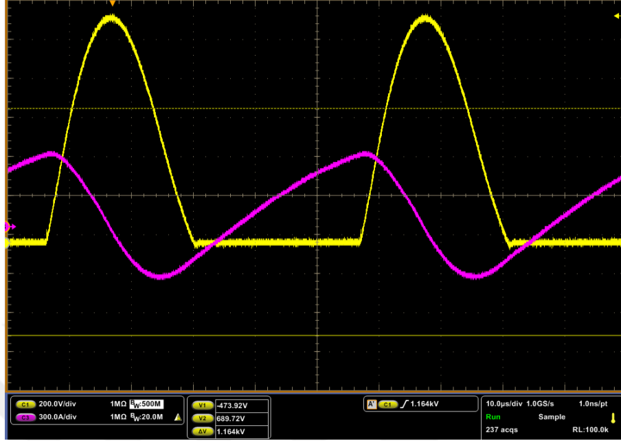
Figure 58: IGBT Collector-Emitter Voltage and Coil Current
