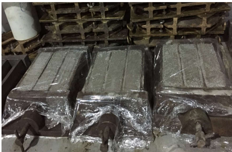
Figure 3.19 Standard Three-Gang Molds
