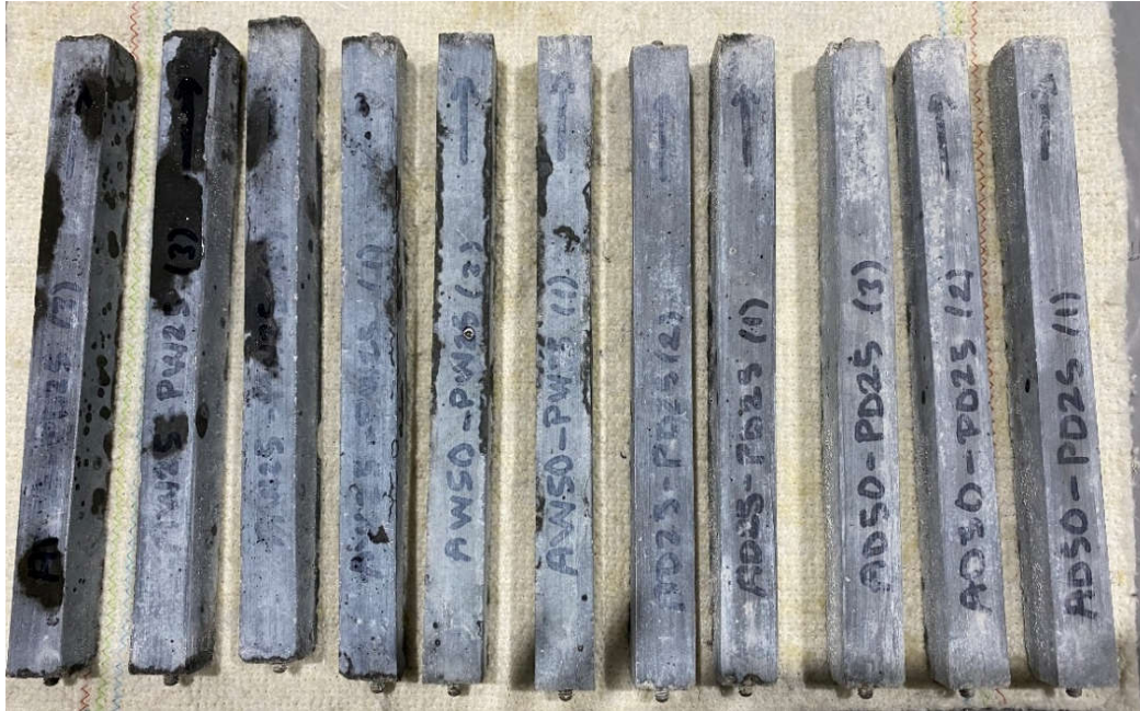
Figure 4.28 ASR Map Cracking Formation of Part Three Mixtures
