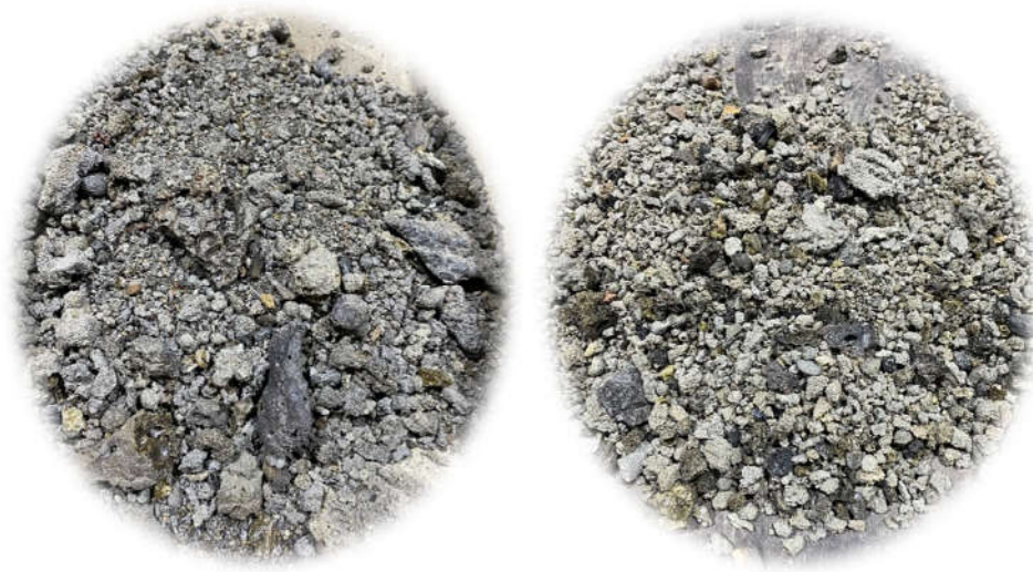
Figure 3.1. Dry-Handled Bottom Ash & Wet-Handled Bottom Ash, Respectively
