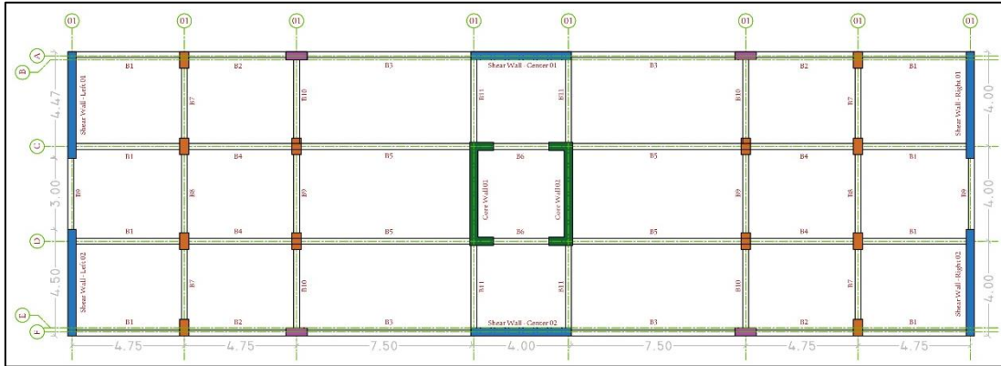
Figure 4.1: 1 st to 5 th Floor Plan.
