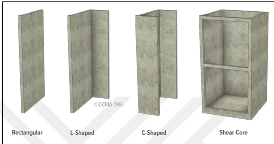
Figure 1.5: Shear wall (CCPIA.ORG).
