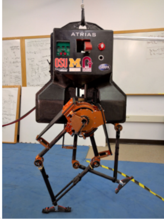
Figure 5.1: Carnegie Mellon University's copy of ATRIAS bipedal robot designed and built by Dynamic Robotics Laboratory at Oregon State University [46].
