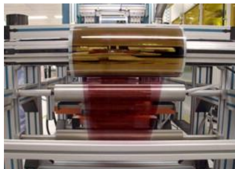
Figure 1.3 Example of a roll-to-roll coated OPV device on a PET foil (Polyethylene Terephthalate) substrate [6]. Copyright 2011 by Elsevier.
