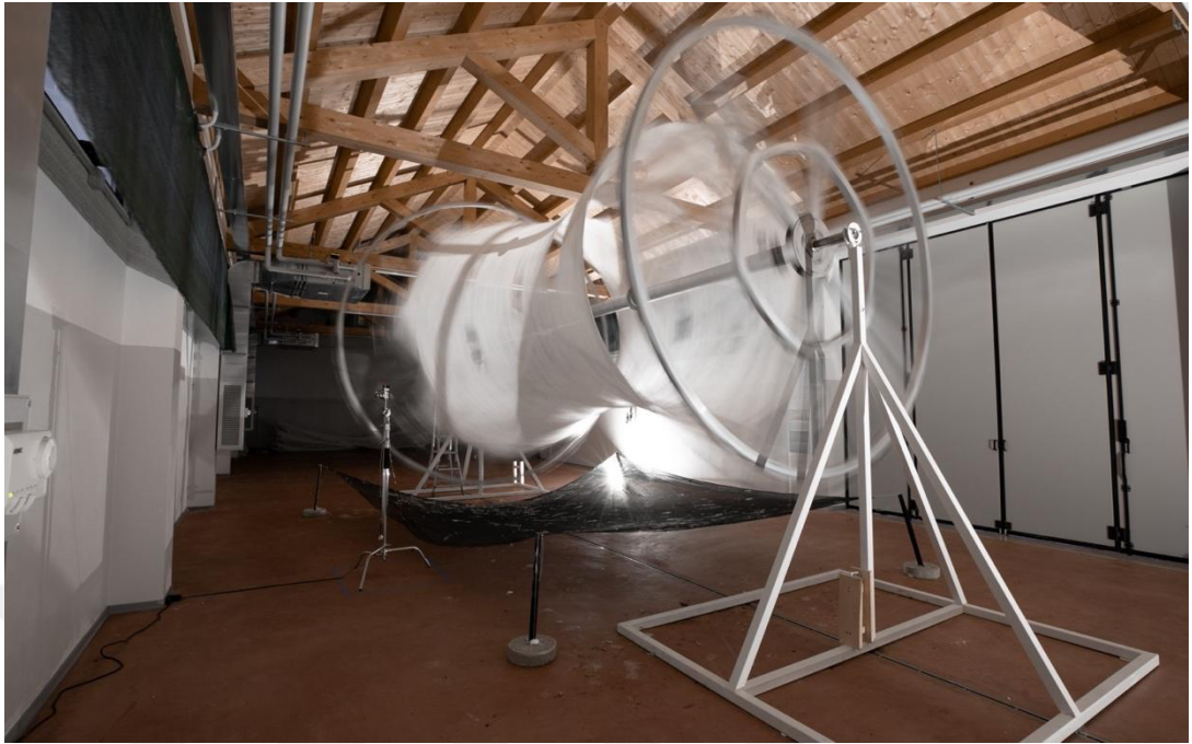
Figure 45 - Long exposure photograph of rotating jig enabling uniform silk deposition, Neri Oxman and Mediated Matter
