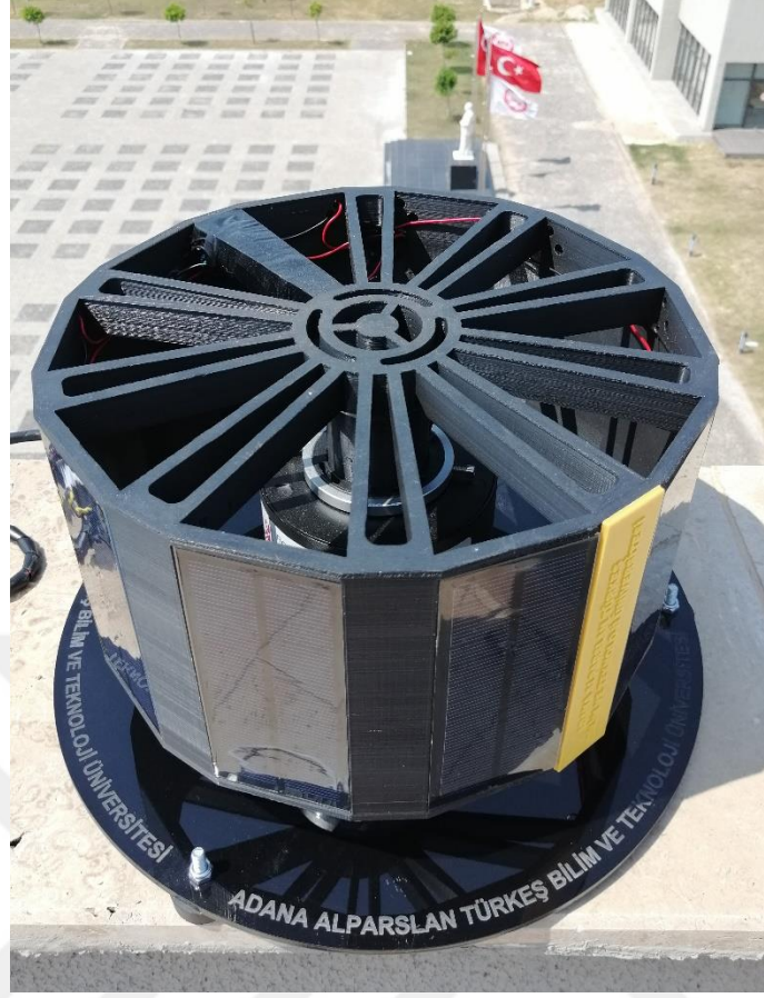
Figure 5.6. The slip ring, photovoltaic panel and rotary system integration.
