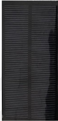
Figure 5.2. The photovoltaic panels in the rotary system.
