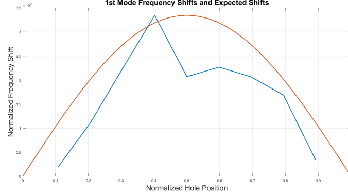
(a) Expected frequency shift profile and experimental frequency shift for the 1st mode
