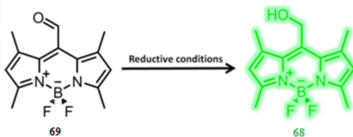
Figure 59: Chemical structure of a hypoxia sensing BODIPY dye.
