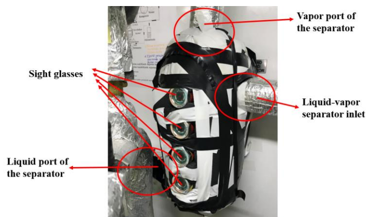
Figure 8.5 Inlet and outlets of the insulated liquid-vapor separator used in the EERC (Personal archive, 2020)
