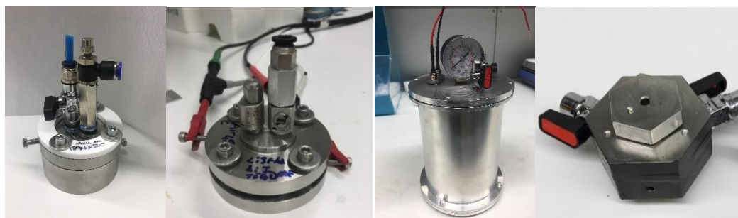
Figure 3. 4. Our own special designed Li-air battery test cells
