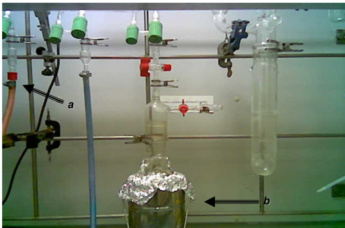
Figure 4.2 a) NH_3 inlet; b) Pyrex reaction tube was placed into liquid nitrogen-ethanol mixture
