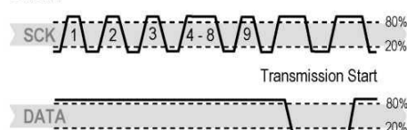
Figure 13: Connection Reset Sequence
