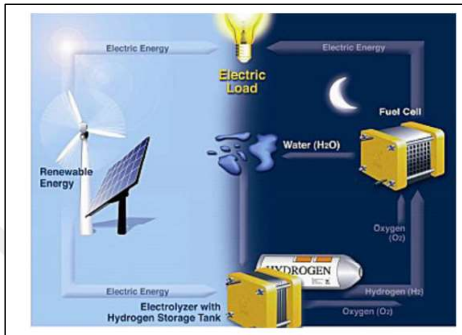
Figure 3.24: Solar Hydrogen Energy Cycle.
