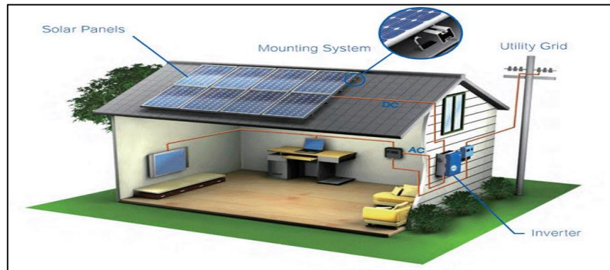
Figure 1.2: Installation of a Photovoltaic System in a Residential Building [8].
