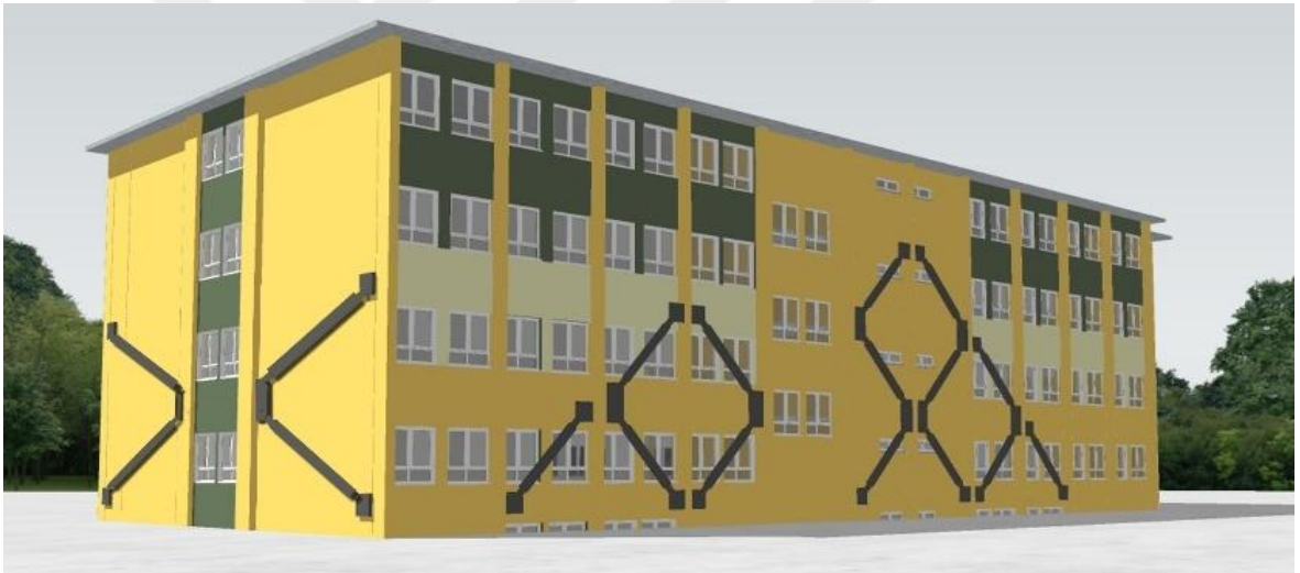
Figure 4.52. 3-D view of the building (representing the retrofitted case with FVDs) formed in Sketch-up Software (cont.).
