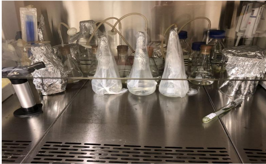
Picture 3.3. Working area under the laminar flow sterilized with ethanol in front of fire gas.
