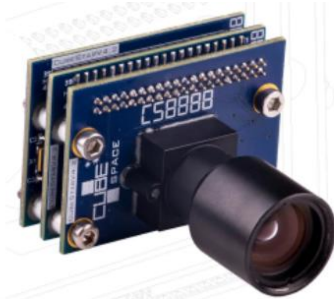
Figure 1.3.1. CubeSat Star Tracker Sensor, CubeStar. [12]
