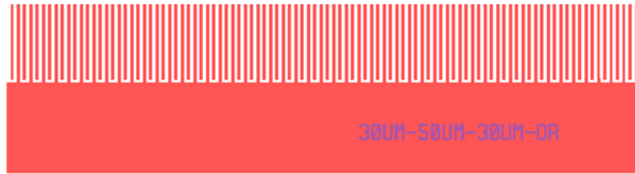
Figure 2.2. Comb-like electrode design for both positive and negative charging.
