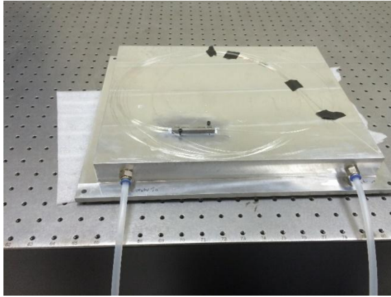
Figure 2. 9: The cooling plate for combiner(produced by Ermaksan)
