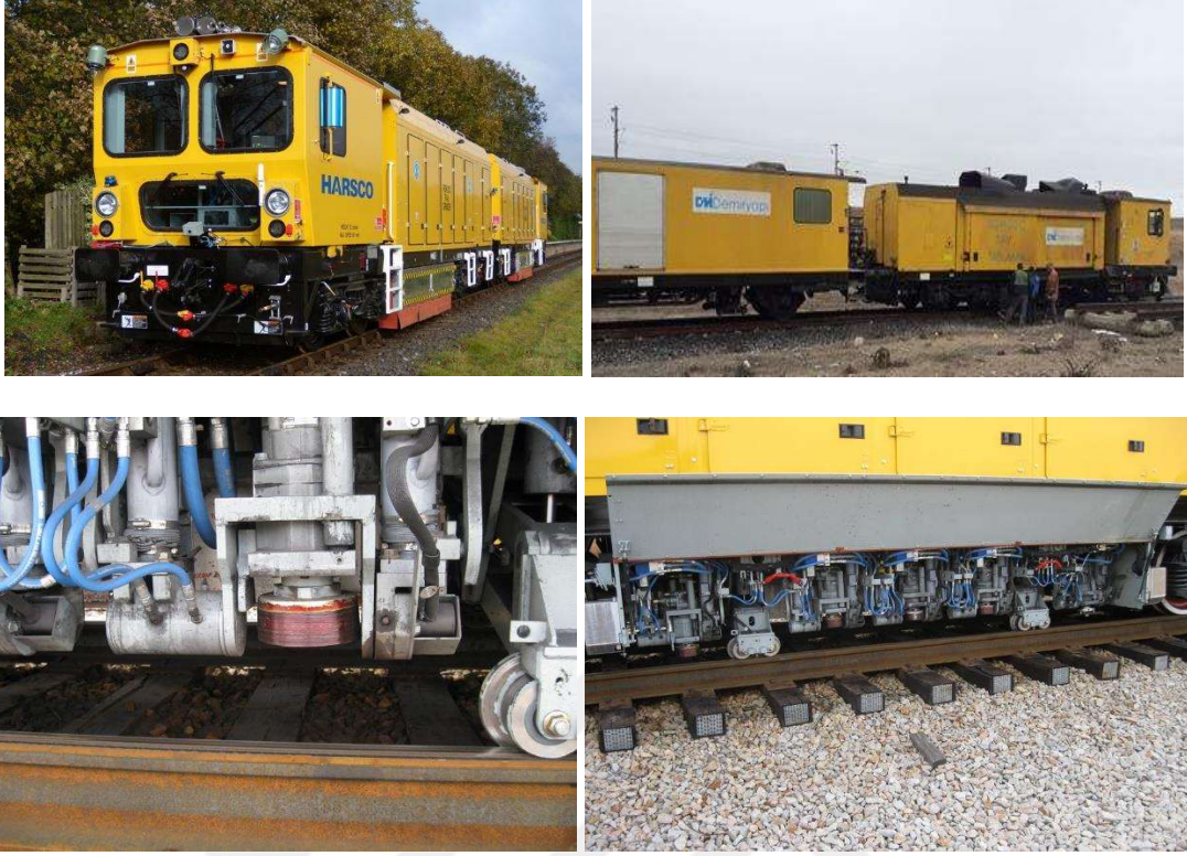
Görsel 2.3. RGH 20 C model taşlama makinesi (railway, 2024)
