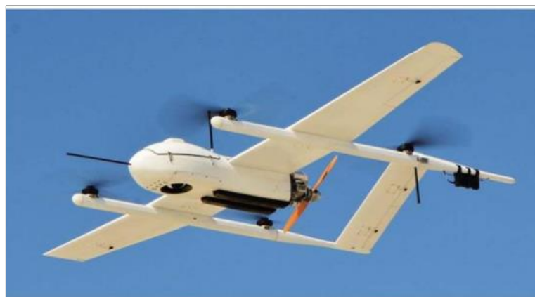
Figure 1.4: Fixed-Wing Hybrid VTOL UAV [7].
