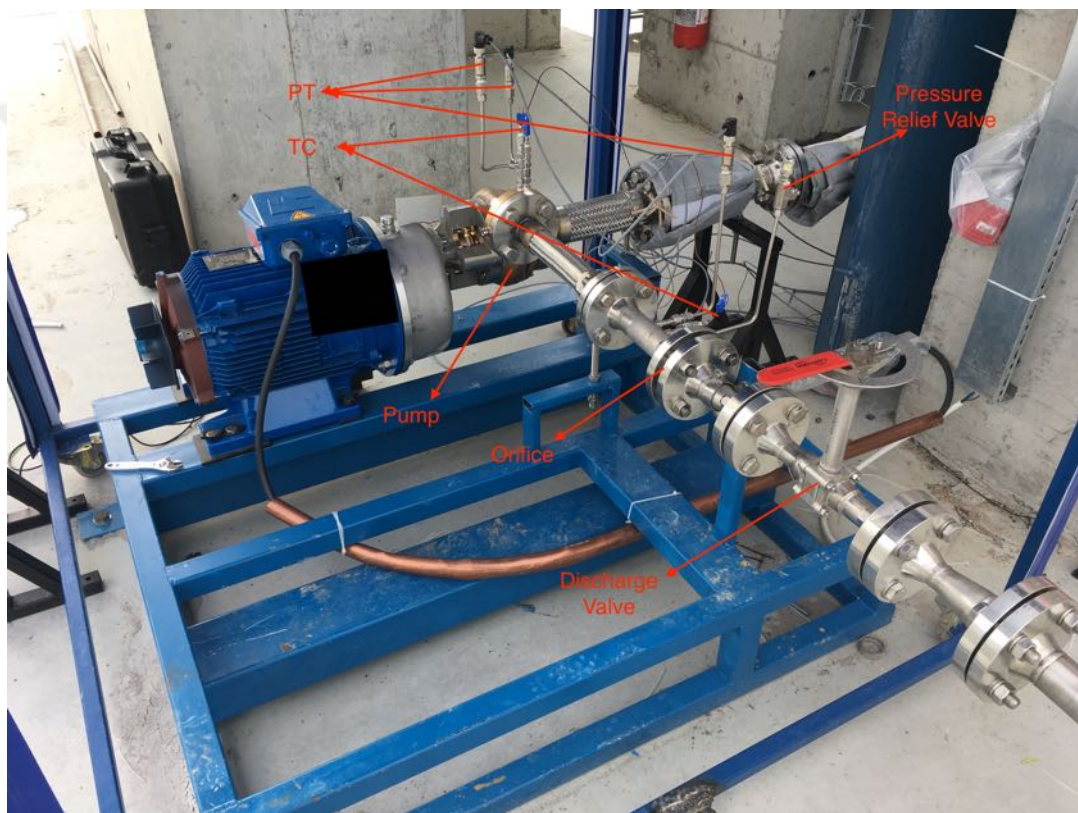
Figure 6.16: Pump test bench, PT = Pressure Transmitter, TC = Thermocouple.
