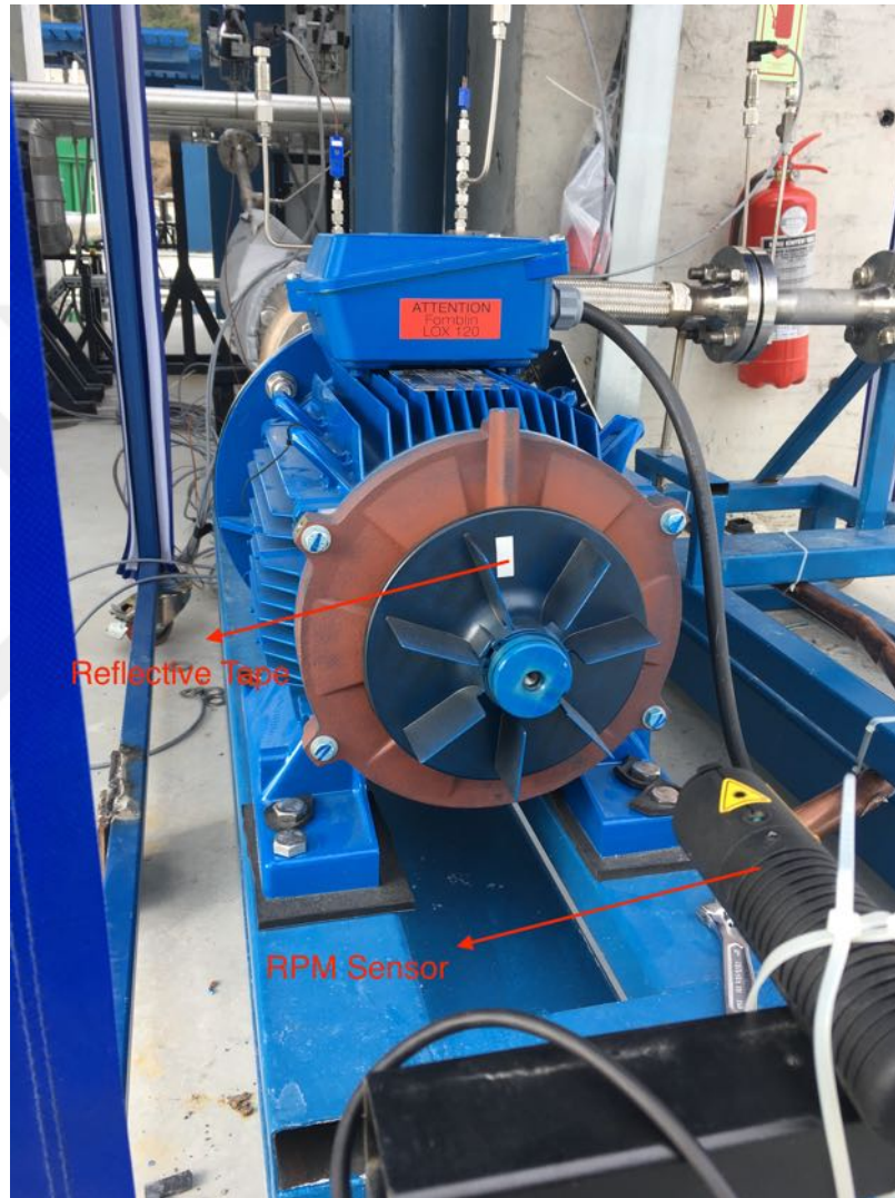
Figure 6.18: RPM Sensor placement on cooling fan.
