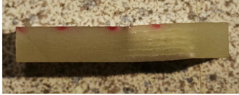
Figure 4.19 - Short beam test specimen after failure
