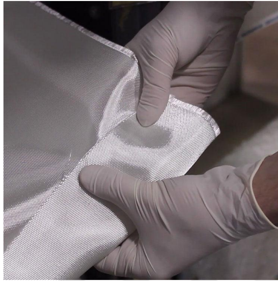
Figure 2.5 - Fibreglast 8HS woven fabric [48]
