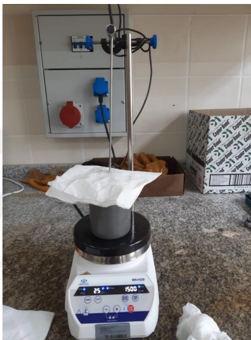
Figure 3.18 Preparation of the ethyl silicate resin & powder mixture (Personal Archive- 2023)
