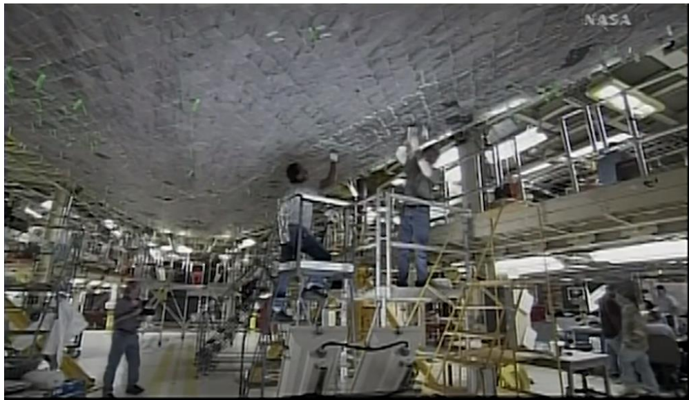
Figure 3.14 Placement of heat tiles on spacecraft (Personal Archive- 2023)
