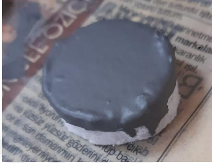
Figure 3.22 Boron carbide & silicon carbide coating sample (Personal Archive- 2023)
