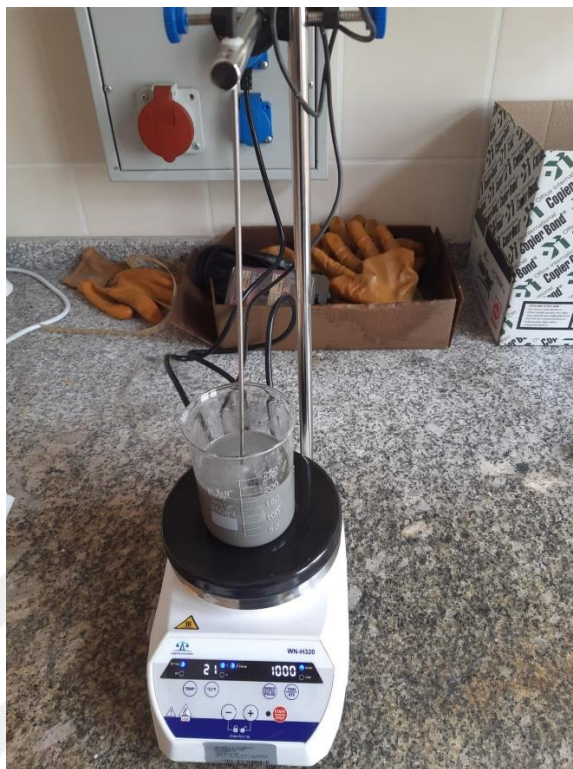
Figure 3.16 Preparation of the ethyl silicate resin and silicon carbide powder mixture (Personal Archive-2023)
