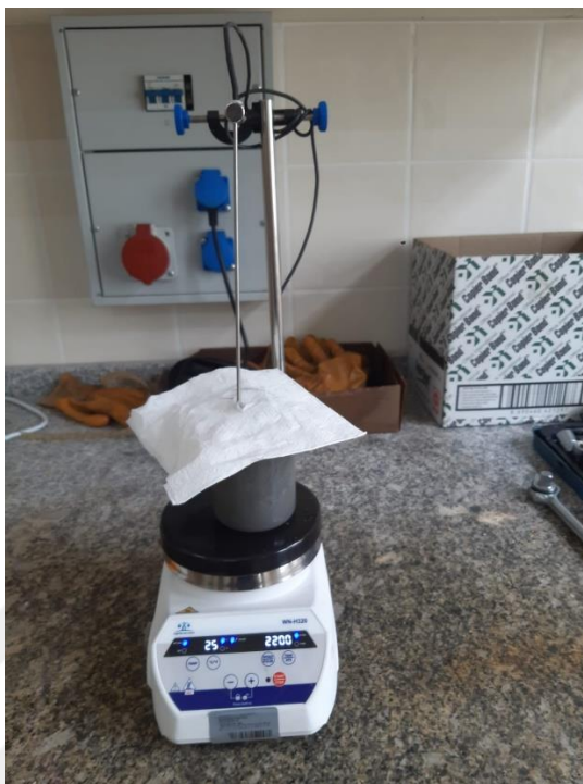
Figure 3.17 Preparation of the ethyl silicate resin and boron carbide powder mixture (Personal Archive-2023)
