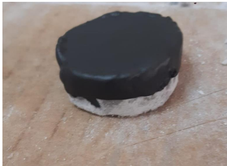
Figure 3.21 Boron carbide coating sample (Personal Archive- 2023)
