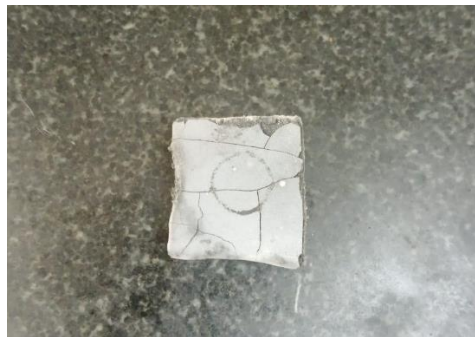
Figure 3.36 Test result of boron carbide coated material (image) (Personal Archive- 2023)
