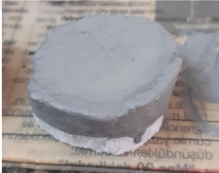
Figure 3.23 Silicon carbide coating sample (Personal Archive- 2023)
