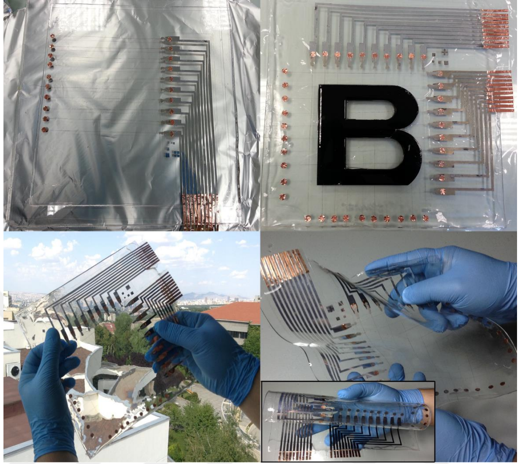
Figure 14. Optical image of fabricated large area electronic skin. Optical images of first and second layer images of electronic skin with letter 'B'. Bottom images demonstrate completed map transparency and flexibility.
