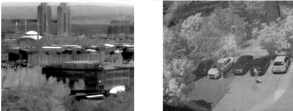
Figure 5.1. Comparison of LWIR (left) [10] and SWIR camera (right) [93] images.
