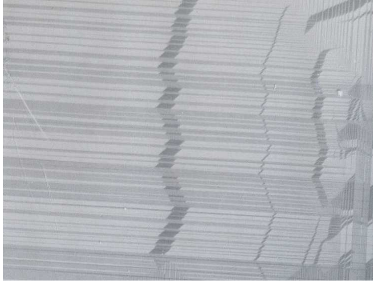
Figure 1.4: 50X magnification photo of LaAlO_3 . The twinning in LaAlO_3 is seen. (Photo by Rizwan Akram.)
