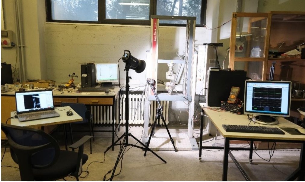
Figure 16. Tensile test and electrical resistance measurements setup.
