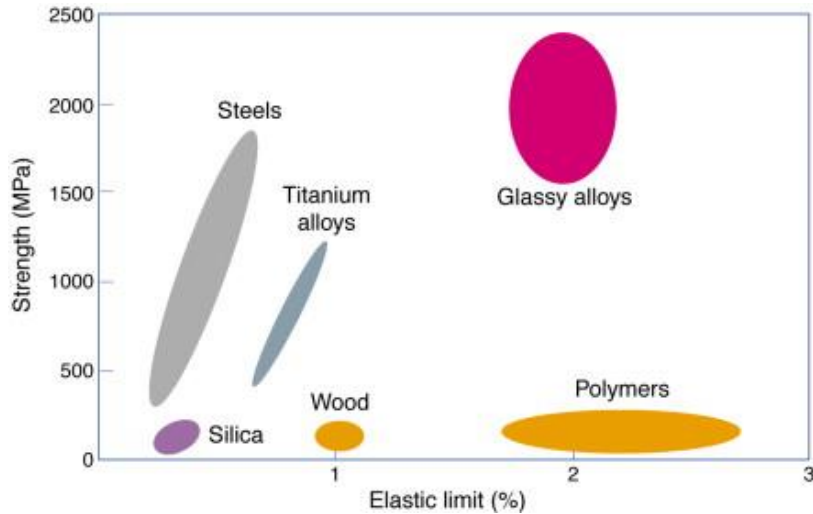
Figure 2. Amorphous metallic alloys combine the superior strength of crystalline metal alloys with the elasticity of polymers [21].
