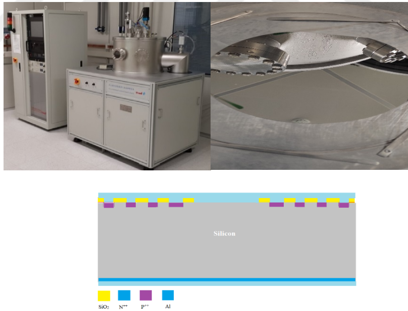
Figure 3.22. The structure formed after the Al coating process
