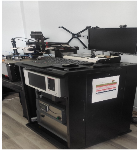
Figure 3.28. Probe station system to measure I-V of Si-PIN PD
