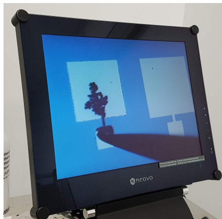
Figure 3.14: Optical image of electrical pads after the insulator broke down.
