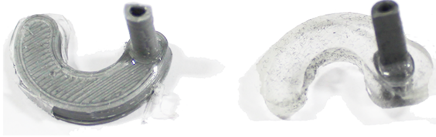
Figure 2.10: C-shaped 3D-printed and PDMS feet with 3D printed cam-shaft extensions.
