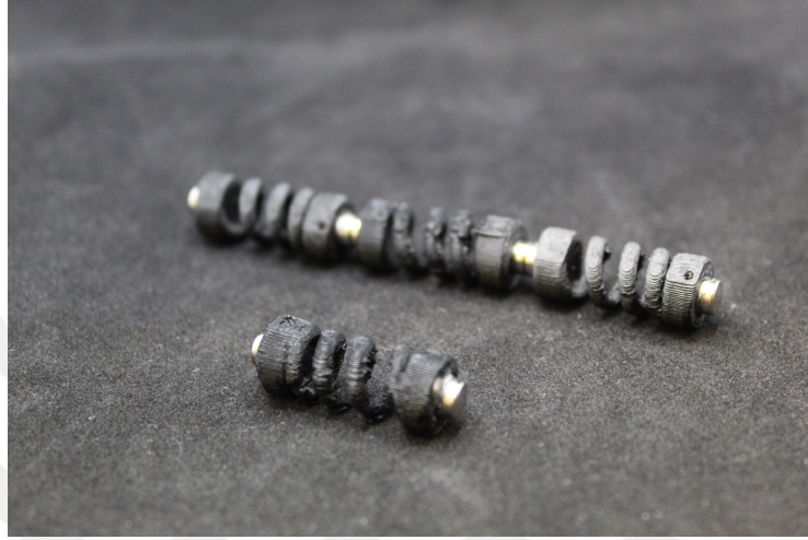
Figure 3.45: The soft coil-shape sensor with varying pitch and magnetic electrical connection.
