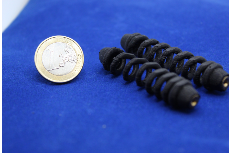
Figure 2.8: 3D printed coil-shaped soft sensors with varying pitch and constant pitch for comparison experiments.
