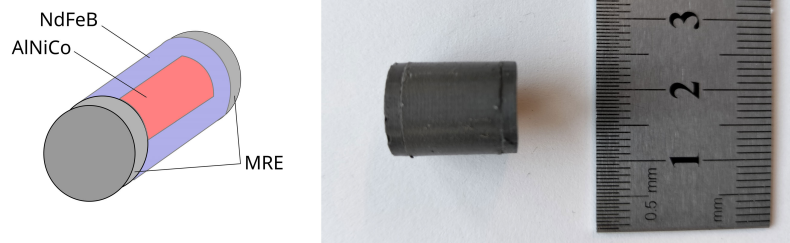
Figure 2.3. Iterated design. The geometry of the srPM is turned into axissymmetric configuration where AlNiCo positioned in the center and outer cylinder is made of NdFeB. The size of the srPM is 16 mm by 12 mm in diameter.
