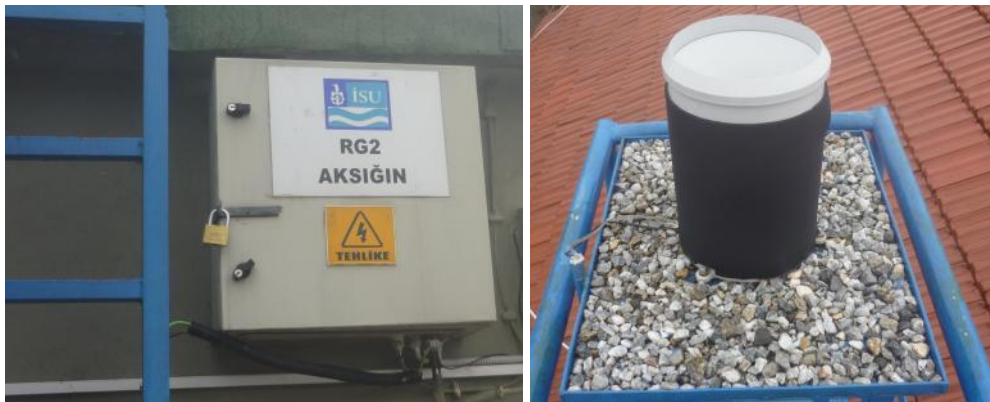
Figure 3.8 Rain-gauge (RG-2) located near at Aksığın village with a heater (320 m)
