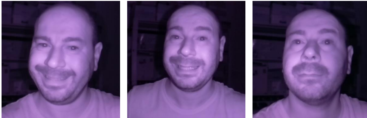
Figure E.2. IR camera capture samples of Dual, Left, and Right illuminated face
