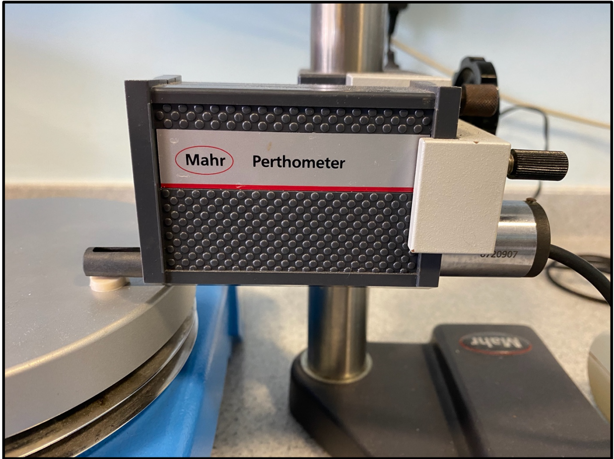
Image 12. The surface roughness measurement of the specimens using the profilometer.
