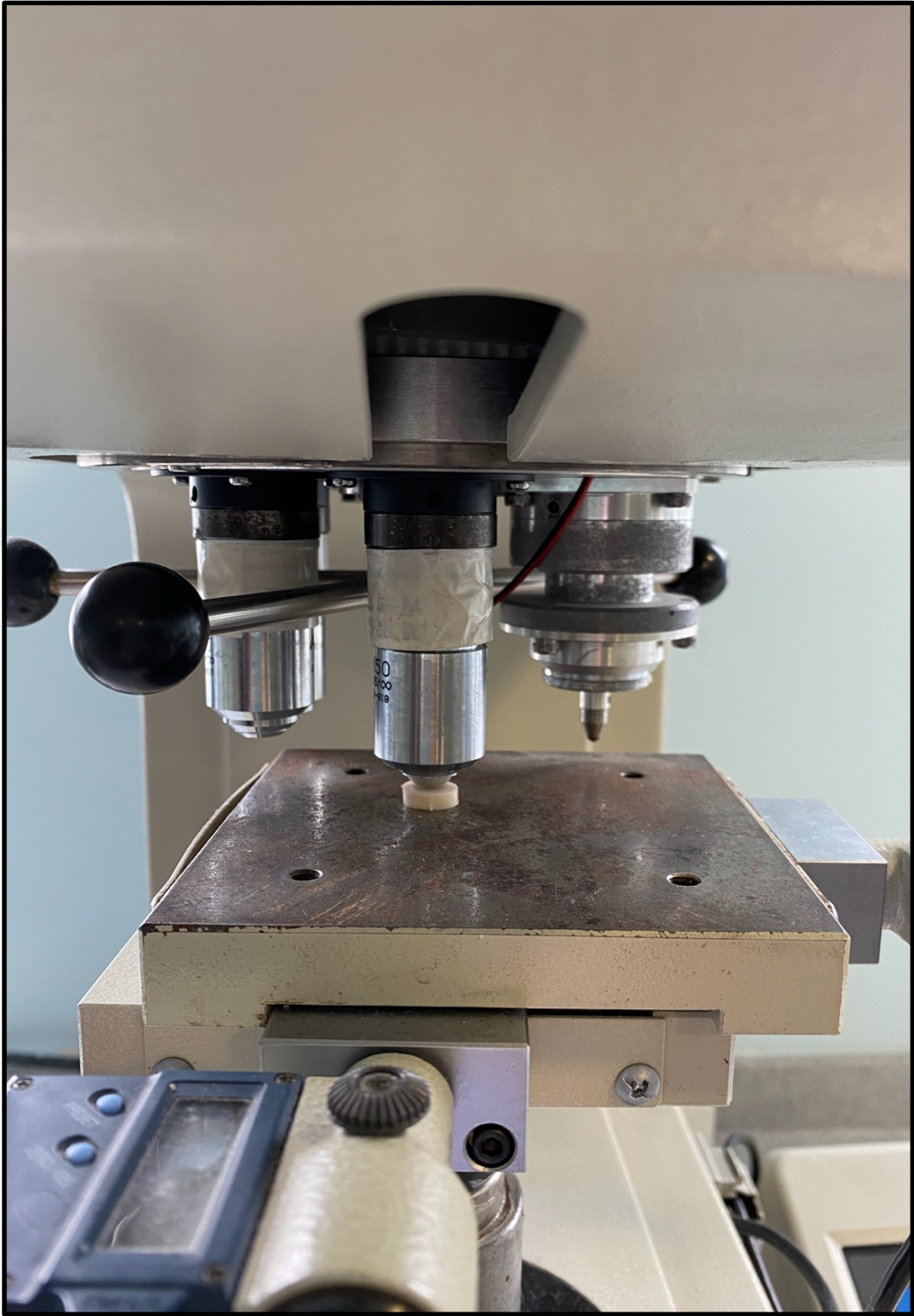
Image 15. Vickers microhardness (VMH) measurements using the microhardness tester.
