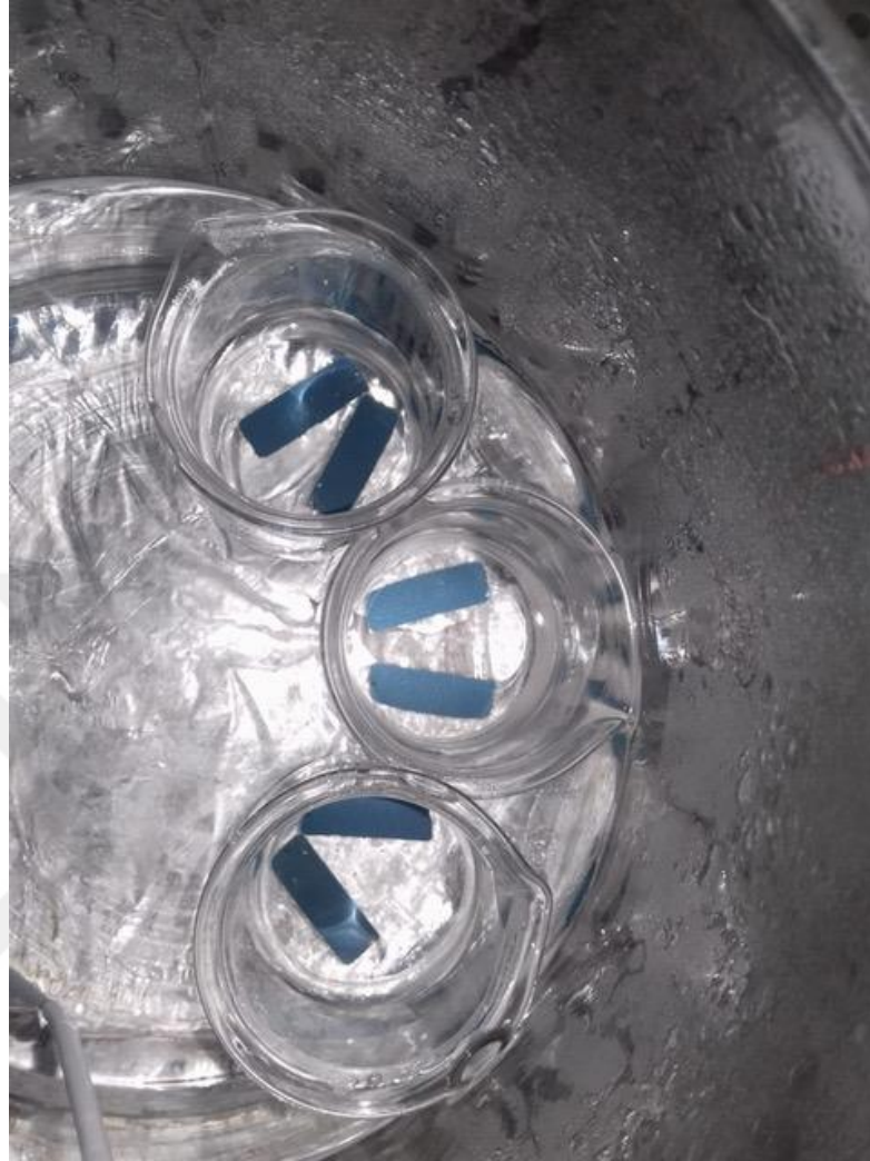
Figure 2.7: This photo is taken from inside the thermal bath with 3 KOH etching flasks floating on top of 65°C water. The best results were achieved by this method instead of using a single layer of thermal control, this ensures the temperature is stable throughout the process.
