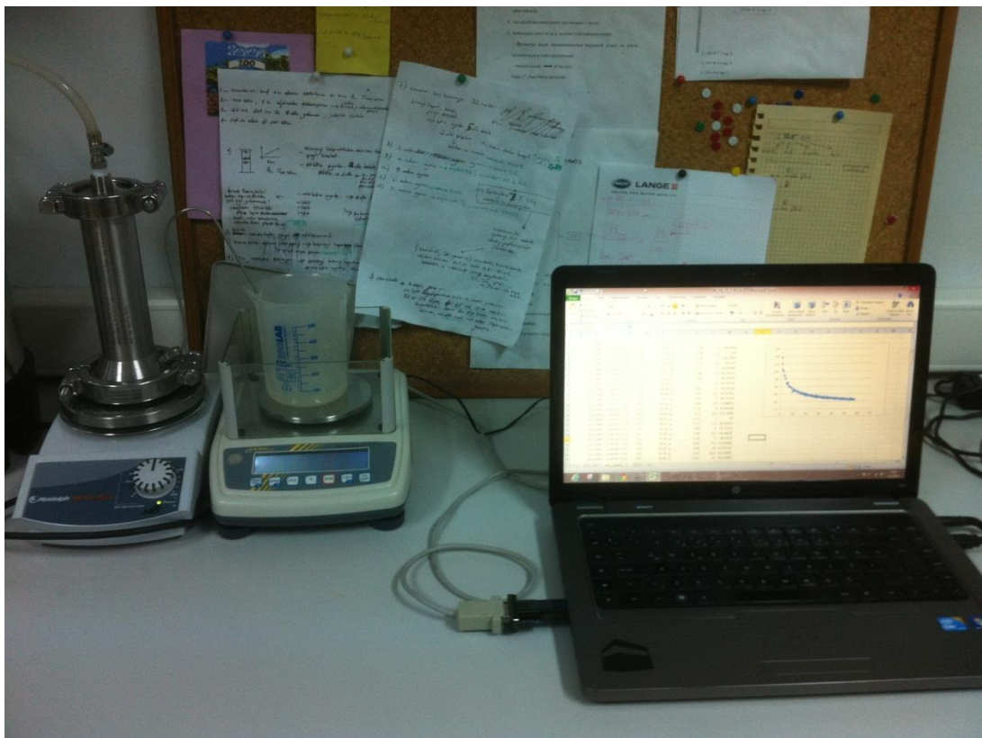
Figure 4.4 : Membrane filtration unit, the weighing device and the computer saving weight periodically for flux measurements.
