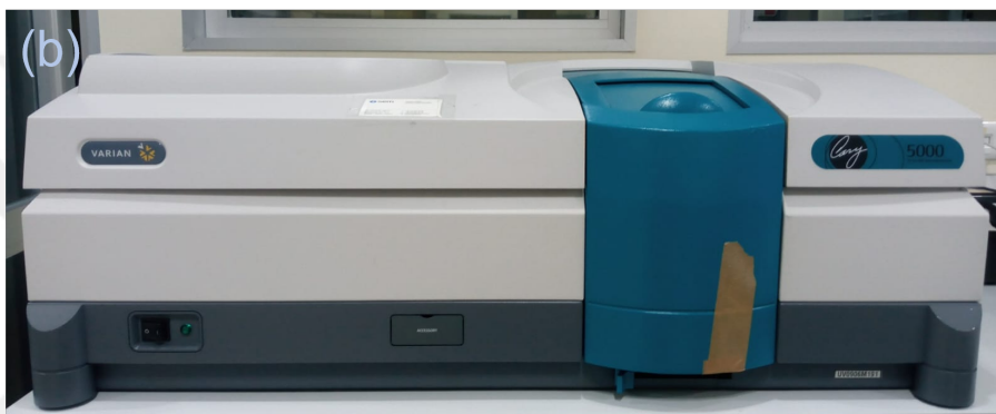
Figure 6.1: (a) Schematic diagram of a UV-Vis spectrophotometer showing the light source, monochromator, sample holder, and detector [6]. (b) Cary 5000 UV-Vis-NIR spectrophotometer used for absorbance and transmission measurements in this study (Cleanroom at Bilkent University, UNAM).
