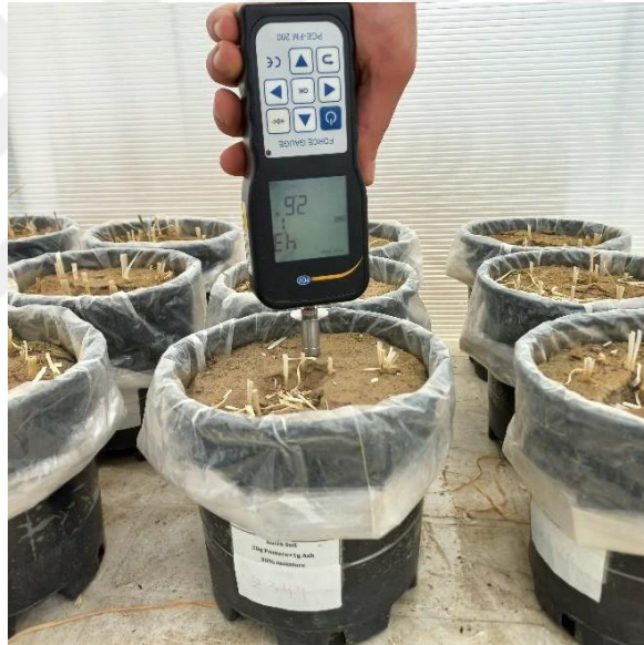
Figure 3.11. Measuring soil penetration resistance in process.
