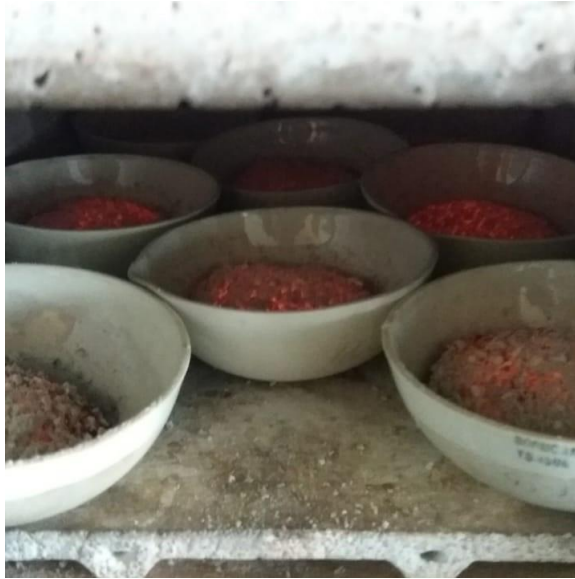
Figure 3.2. Incineration process of OP to produce OPBA.
