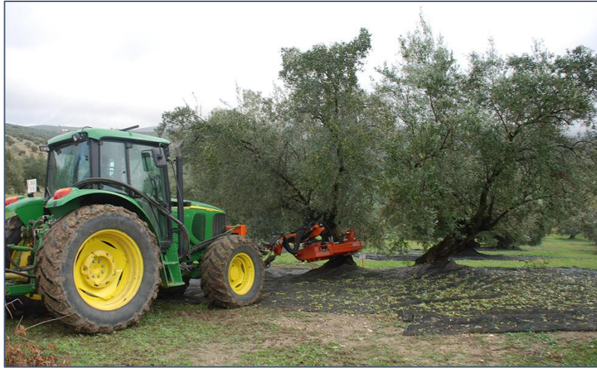
Figure 3.6 Tractor with a trunk shaker (Sola-Guirado et al., 2014)
