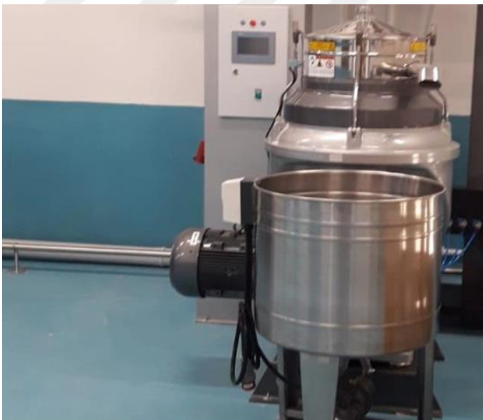
Figure 16: Separator of Malia Olive Oil Mill
