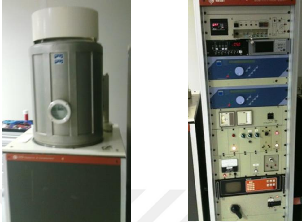
Figure 3.1 Pictures of r.f. magnetron sputtering system
