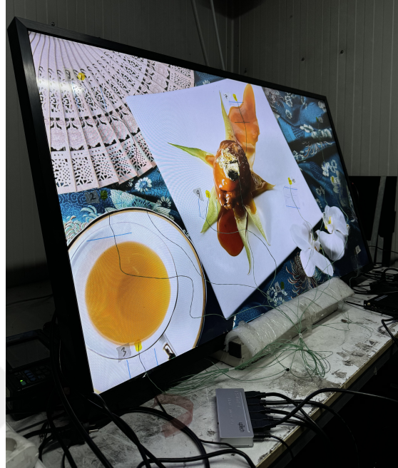
Figure 19: Image of the product placed in the heat room for testing.
