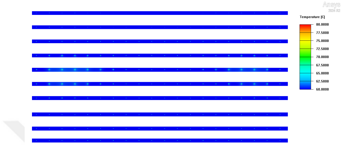
Figure 34: Numerical results for temperature distribution of LED PCBs and LEDs of the product with heuristic cooling system.
