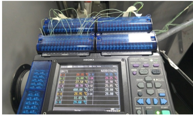
Figure 14: HIOKI LR8401 brand multichannel data logger for thermocouple readings.
