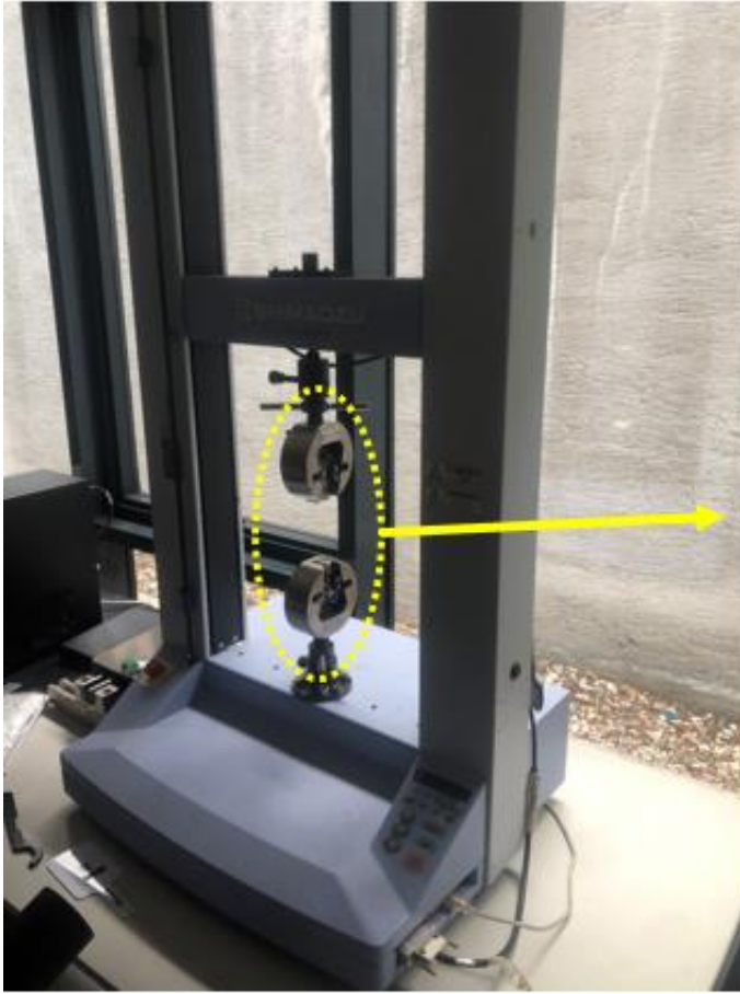
Figure 4.3 10 kN universal Shimadzu AGS-X and schematic representation of universal tensile testing machine (on the right)
