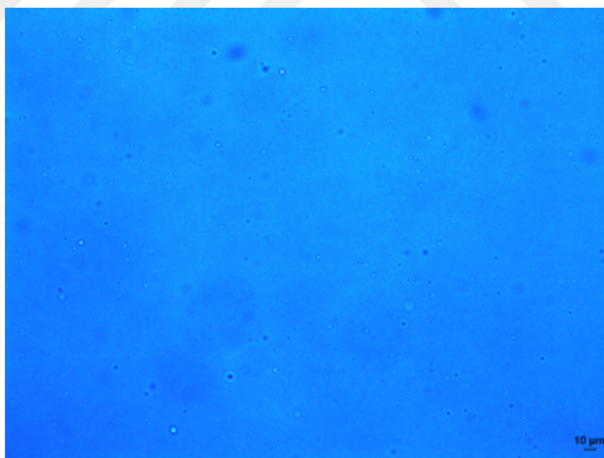
Figure A. 28. Optical light microscopy images of HA-CHI mixture at pH 4.0 acetate buffer solution with 0.15M ionic strength.
